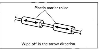
9 After opening the back door by holding down the back door release, following the same procedure as in step 4, use the accessory roller cleaning paper to wipe the surfaces of the rubber carrier rollers and plastic carrier rollers all the way around them proceeding from one end to the other in the directions of the arrows shown in the diagram to the right. Then close the back door.
